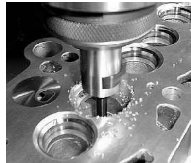
Picture 5 - Cutting the counter bore
